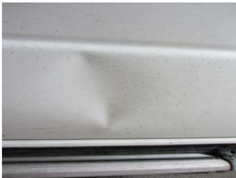
Fig 2.3 Damage to passenger cabin side door
