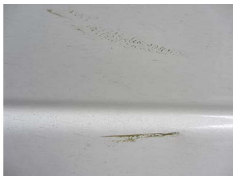
Fig 2.5 Paint transfer to passenger side rear panel
