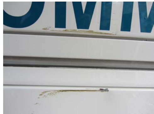
Fig 2.4 Paint transfer to passenger side rear panel
