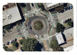
A roundabout with protected bicycle lanes is intended to separate cyclists from vehicular traffic and allocated priority to pedestrians and cyclists at the intersection. This treatment includes raised pedestrian and cyclist crossings on each leg and separated off-road bicycle lanes surrounding the intersection.
