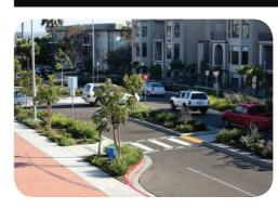
A kerb outstand zebra crossing is intended to allocate priority to crossing pedestrians and reduce vehicle speeds. The treatment comprises of the same components as the wombat crossing, except the crossing is not raised.
