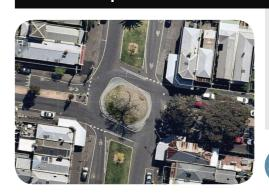
A C-roundabout is a modified roundabout where the central island is of an irregular shape to increase deflection through the roundabout, slow vehicle speeds and increase cyclist safety. This treatment may also include narrow traffic lanes, bicycle sharrows, raised platforms and bicycle signage on the approaches.
