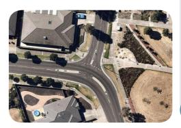
A reverse priority treatment is intended to allocate priority at a T-intersection (or cross intersection) to turning traffic rather than traffic travelling straight along the roadway. This is usually in response to high volumes performing the turning movement. This treatment comprises linemarking and may include kerb outstands and/or traffic islands to reinforce the priority.
