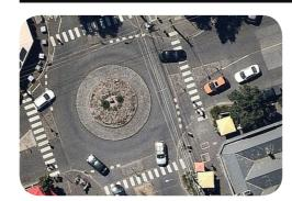
A roundabout with raised platforms on each approach is intended to reduce vehicle speeds and improve pedestrian connectivity at roundabouts.
