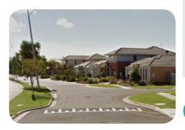
A raised T-intersection is intended to reduce vehicle speeds on all legs at local roads intersections. The treatment comprises a flat top road hump through the intersection to slow vehicular traffic on all approaches. This treatment can include kerb extensions where road width permits.
