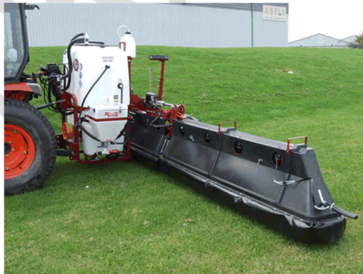
Figure 19. Spray unit with hooded applicator Source: Darebin City Council
