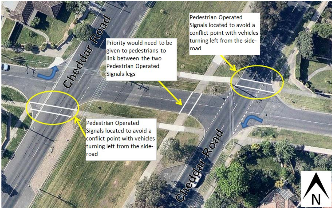
Figure 7: Required 'dog leg' arrangement of Pedestrian Operated Signals at Cheddar Road and a side road
