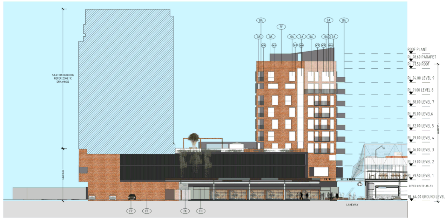
1 Laneway Building Elevation - South SCALE 1:250
