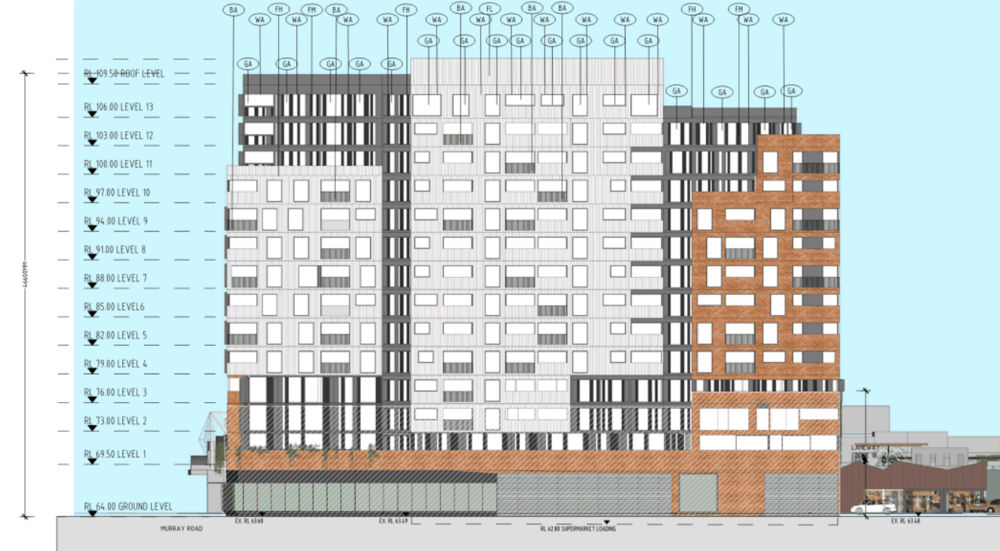
4 Station Building Elevation - West SCALE 1:250
