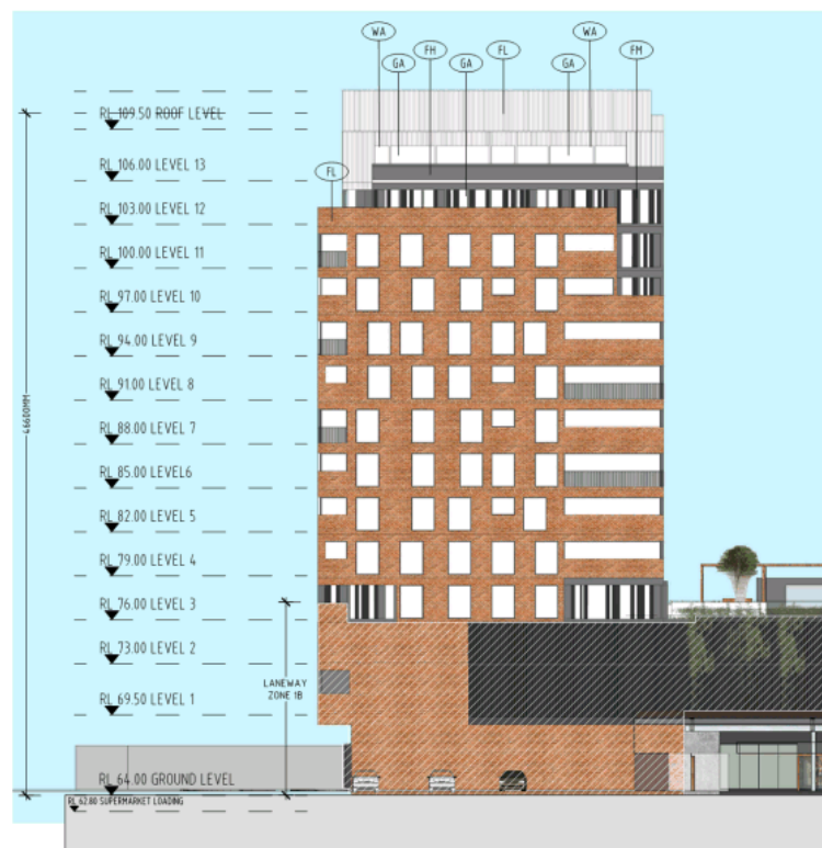
3 Station Building Elevation - South SCALE 1:250
