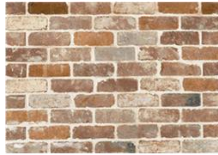
P1 -RECYCLED PRESSED RED BRICK FLUSH MORTAR JOINT LOCATION -LOWER LEVEL WALLS -FRONT FENCE FEATURES
