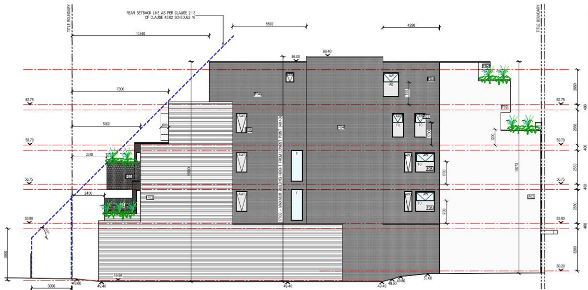
Diagram E: South Elevation showing 45 degree rear building envelope and maximum 17 metre building height.
