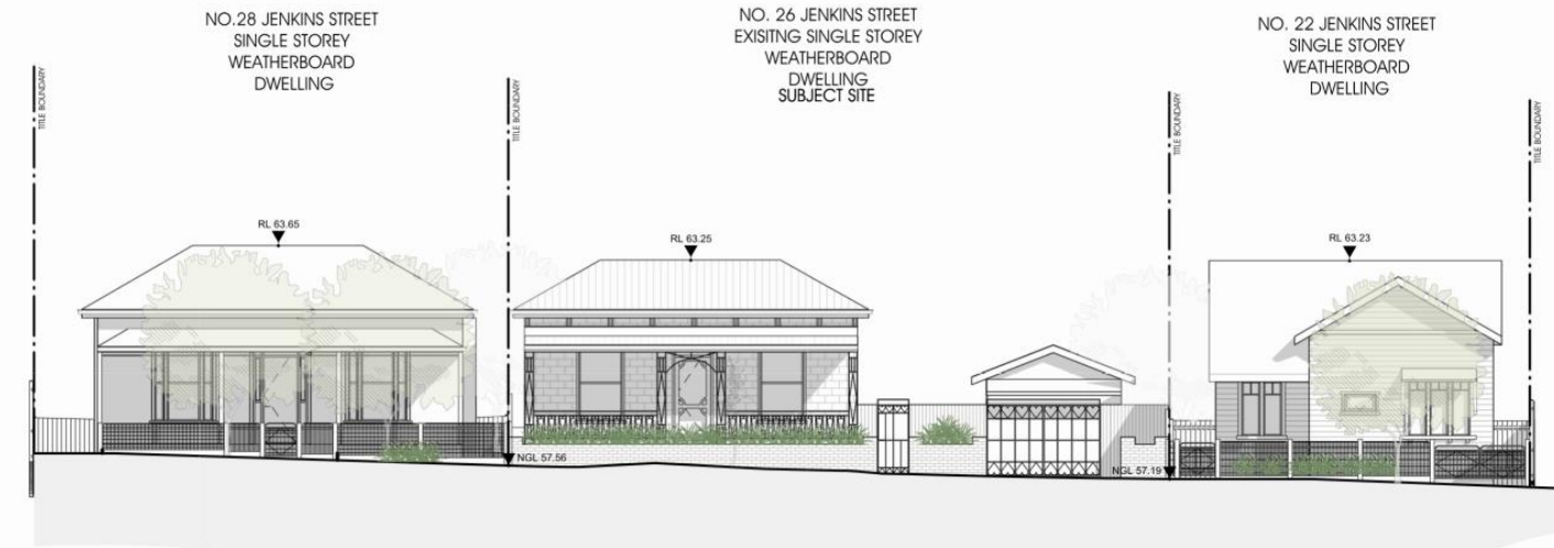
EXISTING STREETSCAPE ELEVATION SCALE 1 : 100
