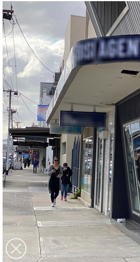
Awnings that are not wide enough do not provide the adequate weather protection.
