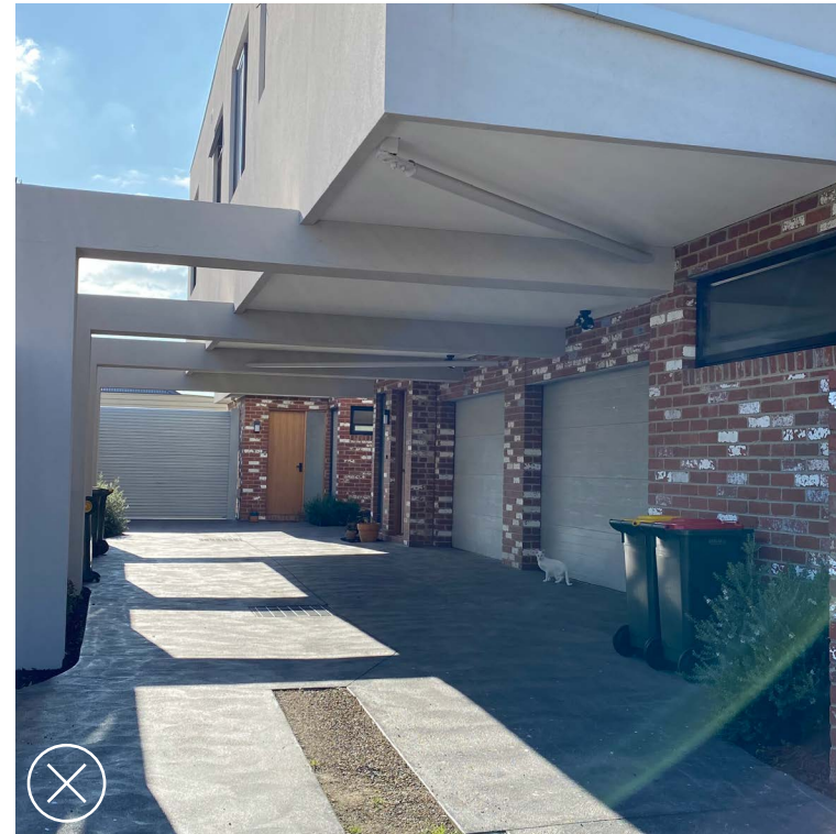
A concrete driveway dominated by garage doors and overhanging building creates a harsh environment and unwelcoming entry to the dwellings.
